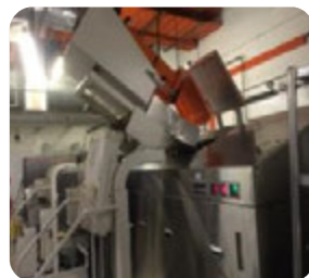
BioHitech Eco-Safe digester
